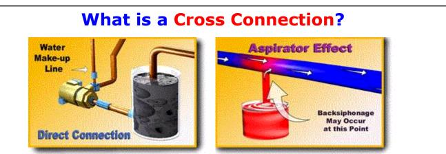
A cross connection is any actual or potential physical connection between a potable water line and any pipe, vessel, or machine containing a non potable fluid, or has the possibility of containing a non potable fluid, solid or gas, such that it is possible for the non potable fluid, solid or gas to enter the potable water system by backflow.
